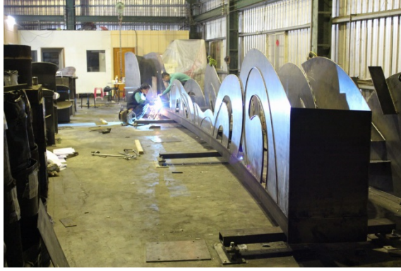
造型焊接→研磨
