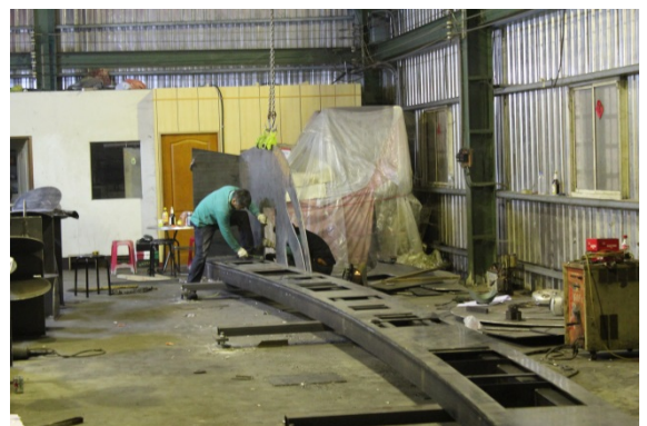
造型焊接→研磨
