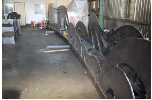
造型焊接→研磨
