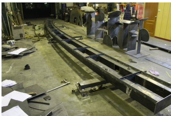
造型焊接→研磨
